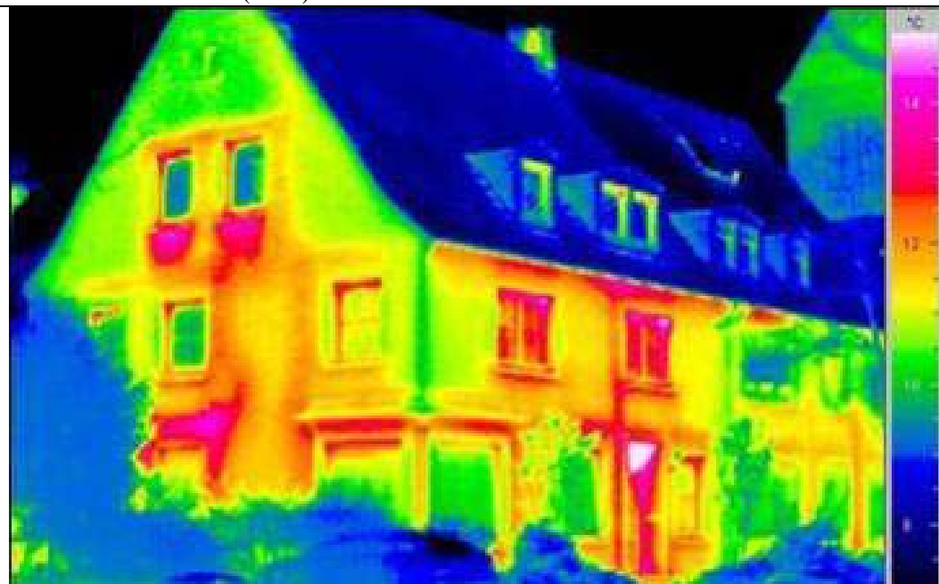
Figure 7.13: Sources of energy losses for a typical commercial building envelope (above), and a thermal image indicating areas of high heat loss (yellow and red areas) from a hotel building
